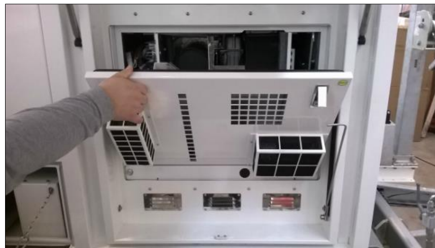
Fig. 12 – Generator rotating panel
