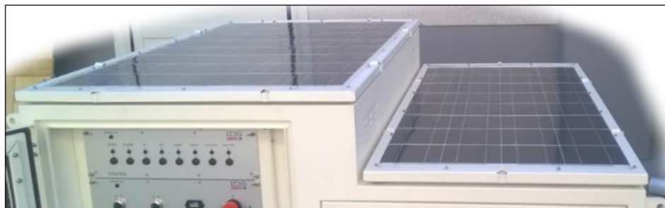
Fig. 27 – ArcSAR Solar panels
